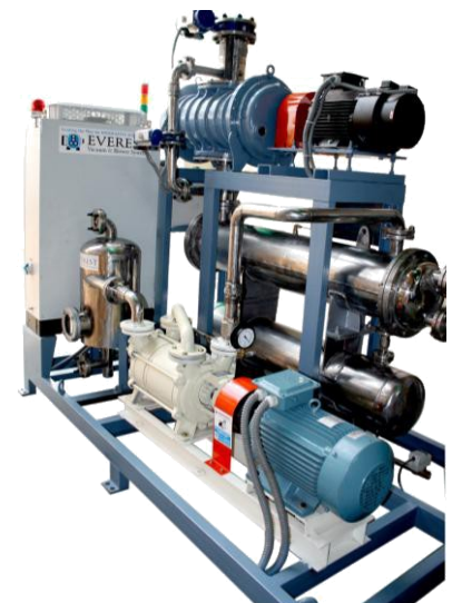
Figure: Water Ring Vacuum Pump+Vacuum Booster
